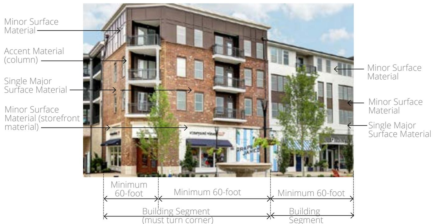
Figure 135-4.1-A. Diagram of Allowed Major Facade, Minor Facade, and Accent Materials
